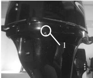
1. Cooling water observation hole
