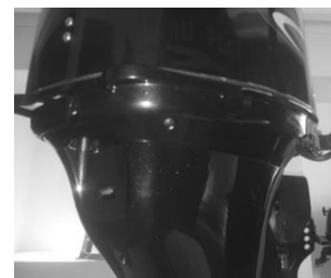
1. Cooling water observation hole
